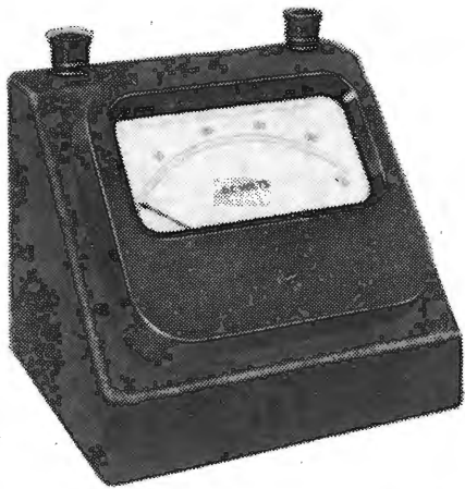
Fig. 23. Example of commercial a.c. thermocouple meter: Taylor "Clarity" Model 42.
